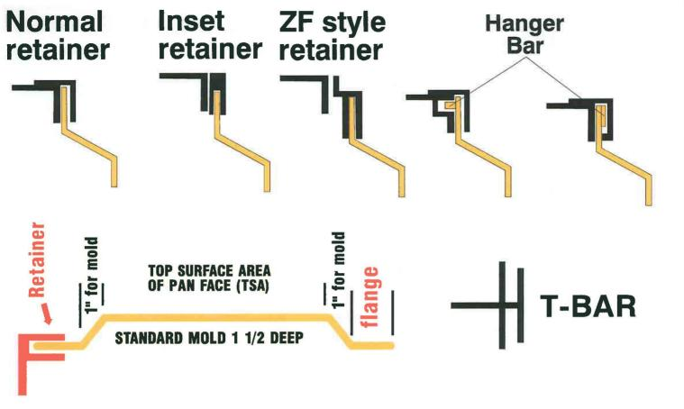
A Flange is the area of a pan face that slides into the retainer A Retainer is an outer piece of metal or aluminum that keeps the pan face from falling out. Pan faces are made from thermoplastic that expands and contracts with temperature changes, about a 1/6 pr foot. It is critical that it be allowed to move back and forth in the retainers as it expands and contracts.
